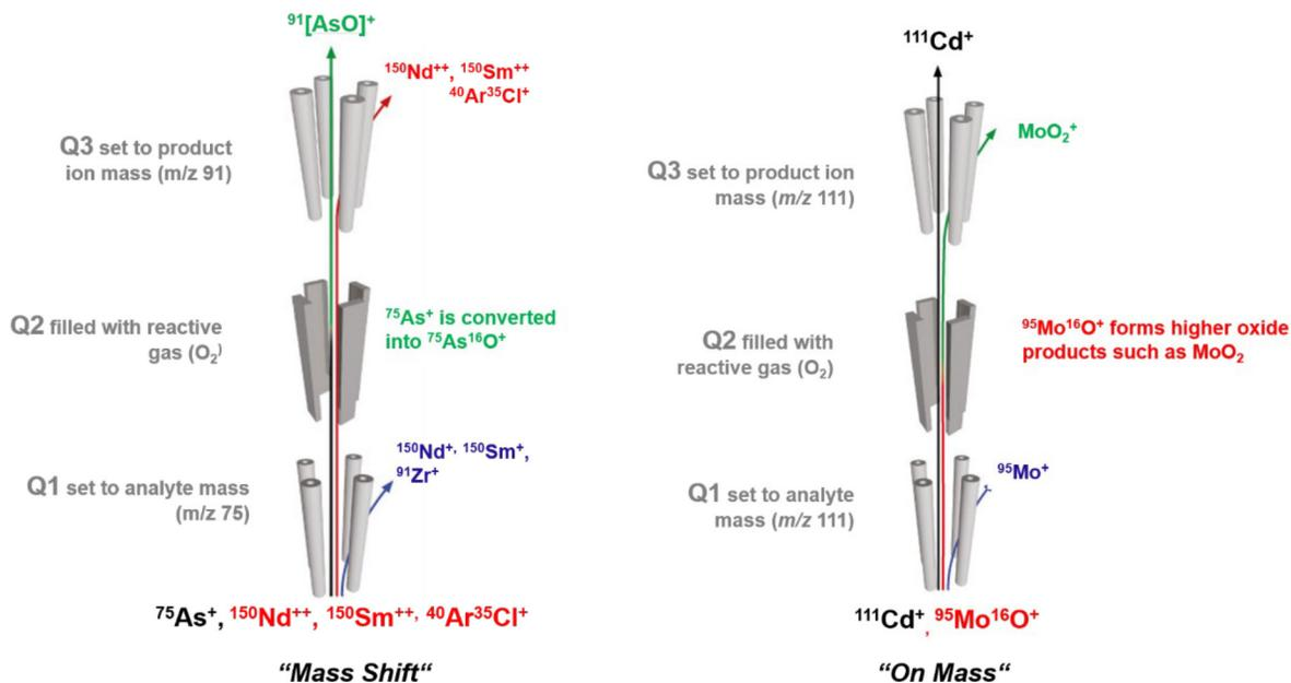
Figure 1. Possible reaction pathways in triple quadrupole ICP-MS
